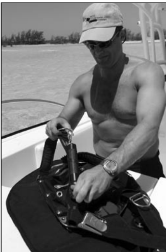
Fig. 8: Cam straps threaded through Pioneer wing and backplate
